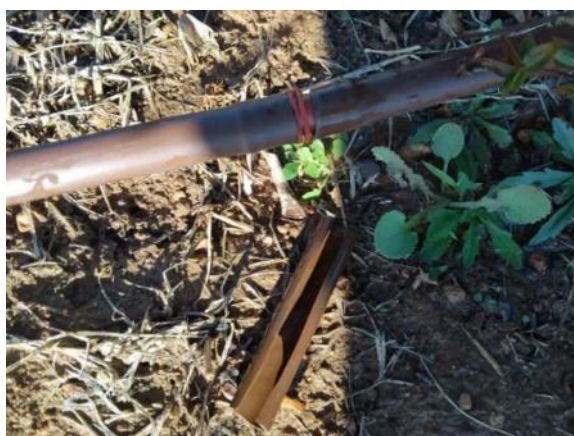
Main road median (4 breaks in PE Ø16-links)
