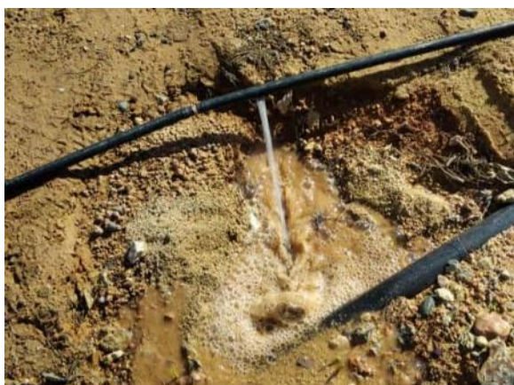
Italian Park Breakage Warning EUC (0,5 ml PE Ø16 and 2 links)
