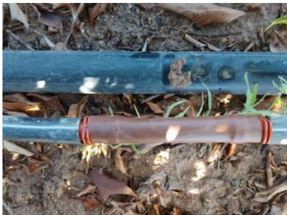
Main road, left side (9 breaks in PE Ø16 - pipe and 2 links)
