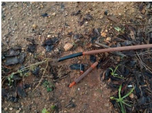
Back garden Phase 6 (5 breaks in PE Ø16-links)
