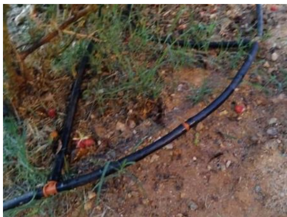
Back garden Phase 6 (5 breaks in PE Ø16- links)
