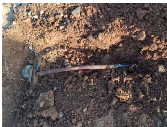
Back garden Phase 6 (5 breaks in PE Ø16-links)
