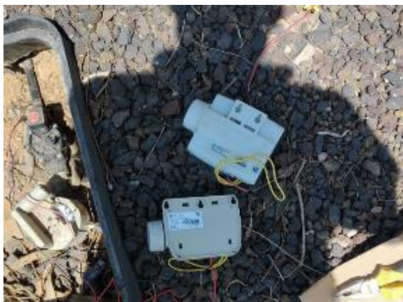
Phase 1 - C/ Germany (replacement of 2 Solem 1E programmers)
